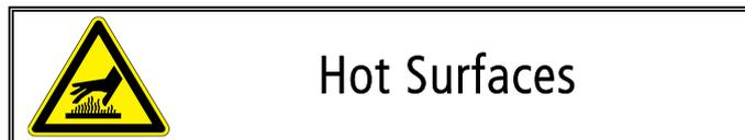
The oven operates internally with hot hair temperatures around 260 °C, therefore there is a risk of burning yourself if not properly operated. Please read this manual, before operating the oven, avoiding this step could cause you serious damages. **Use the Cool Down function to drop the temperatures to a safe level before operating the internal parts.**
