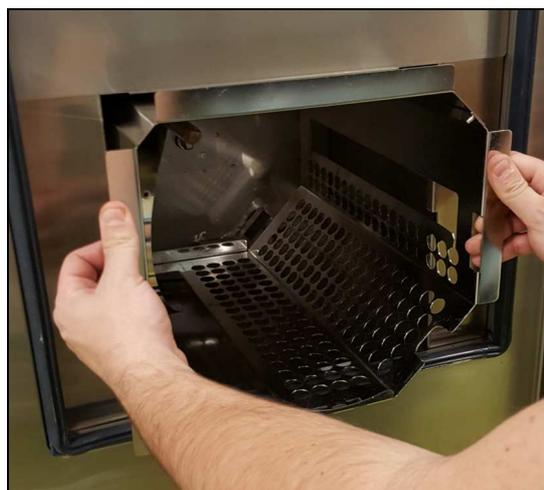
**Figure 25** - Air duct plate pulled halfway out
