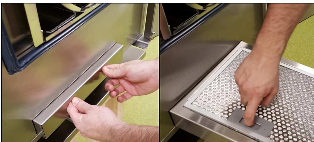
Figure 34 - Air filter partially pulled out
