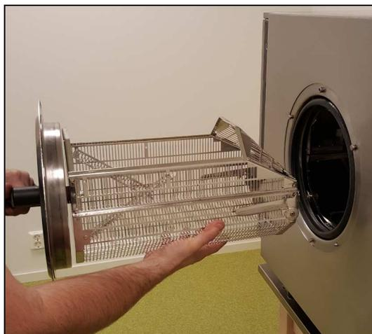
**Figure 21** – Pull out food basket container completely.
