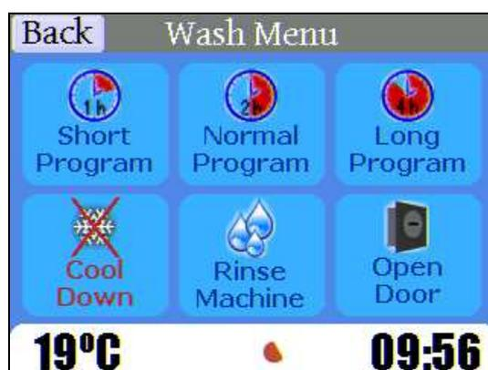
Figure 29 – Screen for selection of dishwasher program or rinse cycle
